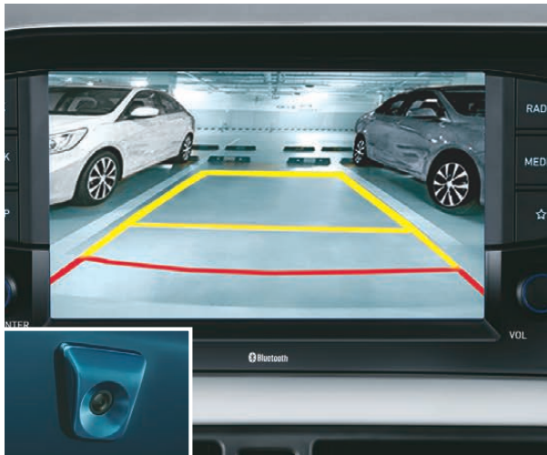
Rear parking camera with display on 20.25 cm screen
